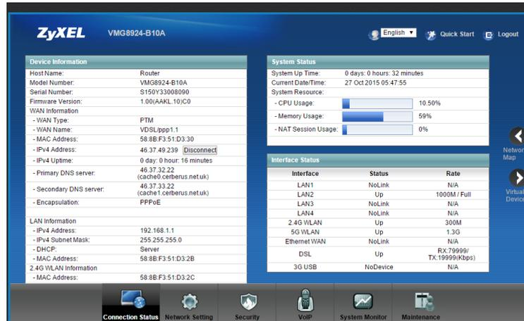
On the left hand side in WAN information you should see that the router has obtained an IP address and DNS server information and has an Uptime which is counting up. In the bottom right hand corner in the Interface status row for DSL you should see status "Up" and see the Sync speed of your line in the Rate Column. Please note that the speed shown is the Maximum possible under ideal conditions. Your speed may be lower based on the quality of your phone line and distance from the Street Cabinet.
